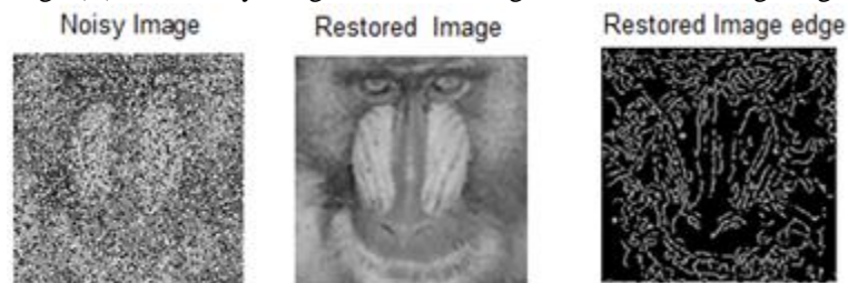
Fig 2(d) 70% Noisy Image, Restored image and Restored Image edge
